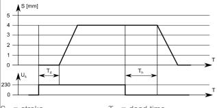
S = stroke $U_s = supply voltage$   $T_d$  = dead time  $T_h$  = hold time
